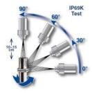
Devices bearing the IP69K rating can be used in applications in which they are exposed to high pressure (1450psi) and high temperature (175°F) wash down
